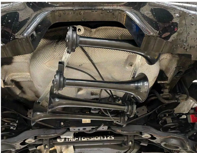
Shocker horns installed underneath a small hatchback.
