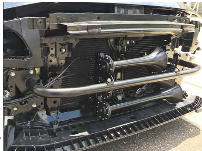
Shocker horns installed in the front grille of a Subaru WRX
