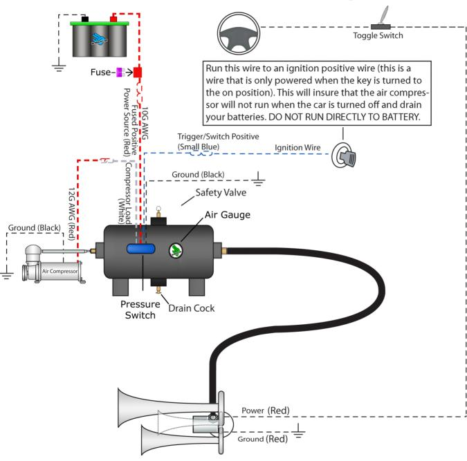
Warning: To ensure the life of your system, reading and following these instructions are recommened. Make sure to change filters and to drain the moisture from the tank on a regular basis. Most factory horns are positively activated. If your horn system is negatively activated, then you will need to wire one of the leads from the valve to a direct 12v power source. Then wire the other lead to the negatively charged horn wire.
