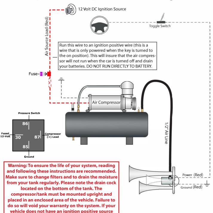
rated for 16AMPs, please use a standard 40AMP relay. If your horn system is negatively activated,
