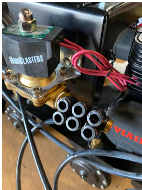
SIX WAY MANIFOLD
