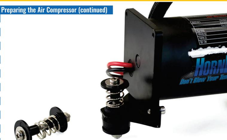
**The 3Q air compressor** features a pair of 3 feet with a spring-loaded rubber mount to reduce the vibration from the compressor while it fills the tank. The feet must be assembled as shown above for the right fit. Do not over tighten these! Finger tight + 1/2 turn is plenty.
