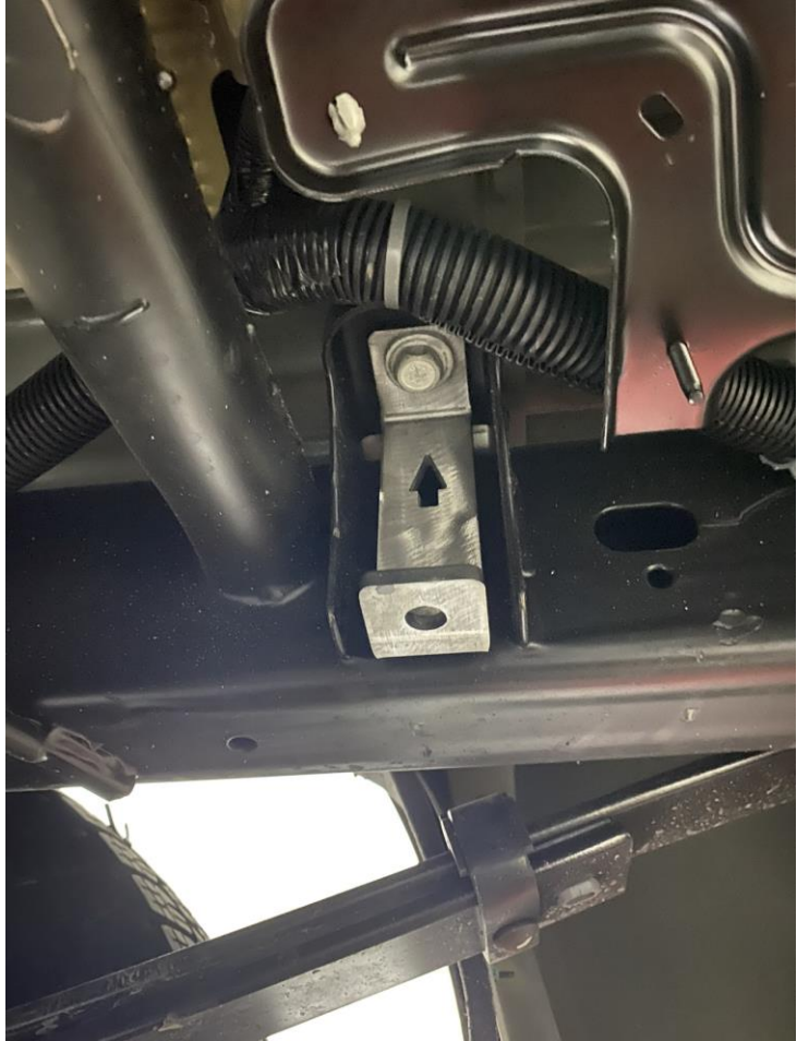
L BRACKET USES FACTORY BODY MOUNT BOLT ON TOP HOLE, ARROW FACING UP LIKE THE PICTURE SHOWS
