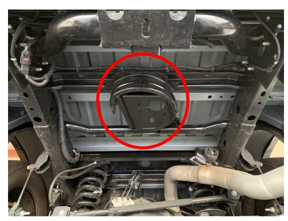
Cut down half circle as far as you can Using a sawzall or cutoff wheel.
