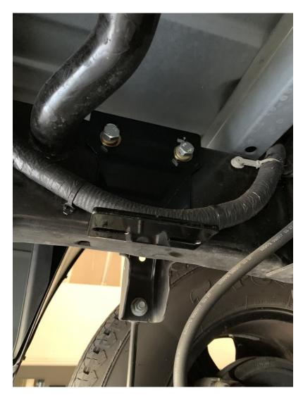
Attach bracket to factory threaded holes using provided hardware. If you have a factory 5<sup>th</sup> wheel, this bracket will not be used.
