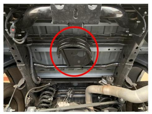
Cut down half circle as far as you can Using a sawzall or cutoff wheel.
