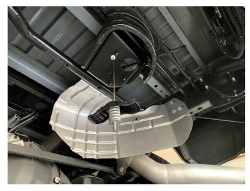
Remove spare tire Remove heatshield Remove spare tire crank assembly
