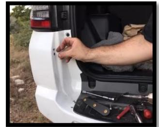
5. Remove the 3 bolts holding the plastic valance in the tire carrier area. This will allow you to gain access behind the bumper.
