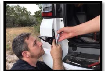
7. Reinstall the Firestik and adjust the mount to ensure it is level and straight.
