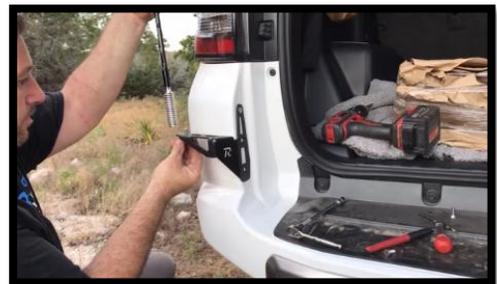
8. Repeat Steps 3-5 for holes 2 and 3. Tighten all holes when complete.
