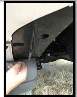
6. Take the mounting plate and reach behind bumper to line it up to the hole. Have a friend help you insert and tighten the first bolt on the mount. Keep it loose for adjustment.
