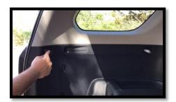
**Step 4**Twist left to remove round tie down knob and unscrew
