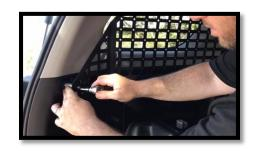
You will want to make sure you lift the weight of the rack to avoid damaging the threads on the spacers when tightening the rack.
