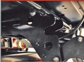
SINGLE CYLINDER LINKAGE MOUNTS ONTO DUAL SLIDE RAILS FOR ULTRA RIGID FRAME AND SIMPLIFIED DESIGN.
