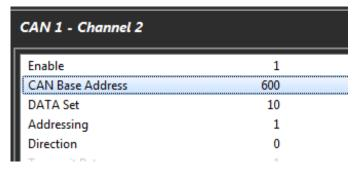
EGT Data is now available on ECU channels "CAN EGT 1 - 4" and Analog data on "CAN AN Volt1 -4" channels.
