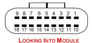
Figure 2.0. Connector Pinout.
