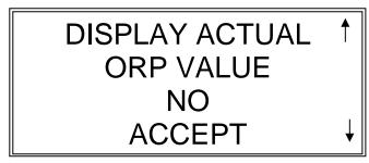
The default value is No, so that during operation the screen will only display "Chlorine OK, Chlorine High or Chlorine Low". Use the arrows up or down to change the default to "YES" and the screen will then display actual ORP levels.
