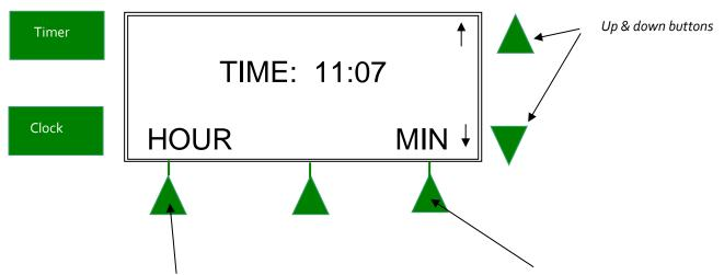
Select hour and use up or down buttons to change hour. Select Min and use up or down buttons to change the minute
