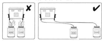
\*\*\*Chemicals MUST be stored apart in accordance with Relevant Standards and Dangerous Goods Codes. Consult your authorized builder or pool shop technician for advice. Chemicals must be at least 1 metre horizontally from control unit in a well ventilated area to avoid corrosive damage.
