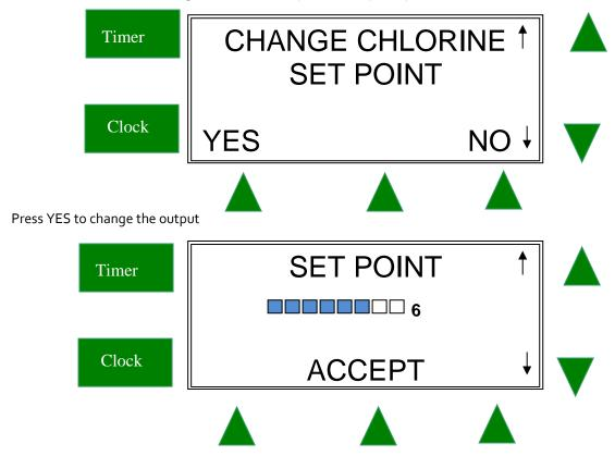
Use the up and down buttons to change the Set Point between o and 8. o chlorine output should only be used when there is no salt in the water. In summer, the chlorine should be set between 6 and 8 and you should regularly check your chlorine level in your swimming pool to determine if the output should be increased or decreased. Rely on your pool professional for advice on the recommended chlorine level in your pool.
