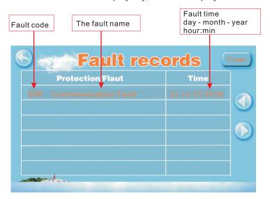
If no failure, main interface displays static " " " " When fault occurs, the fault icon will flash between the " " " " ", the failure interface will record time, code, name of the fault.
