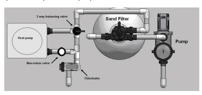
Where the heat pump is installed in the filtration circuit, the heater should always be installed after the pump and filter. The water connections are located on the right hand side of the heater. The inlet and outlet are clearly marked. Water connections supplied are for 50mm PVC glue in plumbing.
