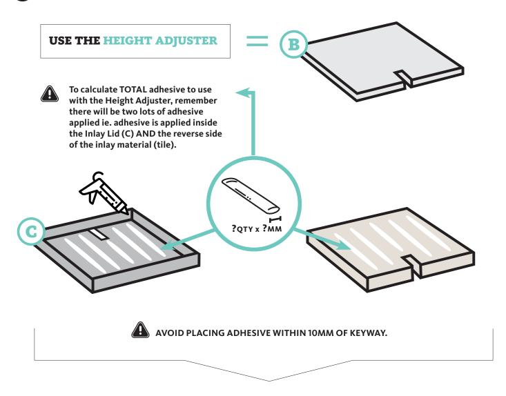
Place Height Adjuster on inlay (tile), then flip Inlay Lid (C) over and press down onto Height Adjuster:
