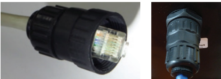
Figure 7.1: RJ45 Plug installed in housing (from rear)
