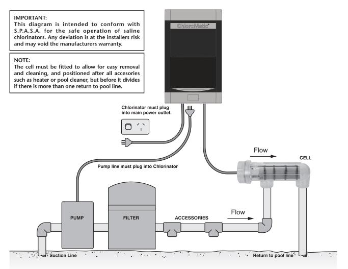
Two self-tapping screws and wall plugs have been provided for fast and simple installation. Simply cut out Template at bottom of page 19 for location of drill entry points. Use a 7mm masonry drill bit when fitting Power Supply to a brick or concrete wall. When mounting to a post drill pilot holes and fit screws provided. Once screws are in position simply hang chlorinator via bracket on back of Unit.
