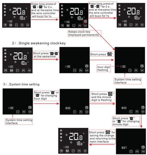
Notes: After the permanent awakening of clock key, if it is not cancelled by user, the main interface will display the clock key permanently. Under the clock setting interface, if short press " " , the change will not be saved and return to the main interface; if there is no operation for 20s, the system will automatically memorize user's setting, and return to the main interface.
