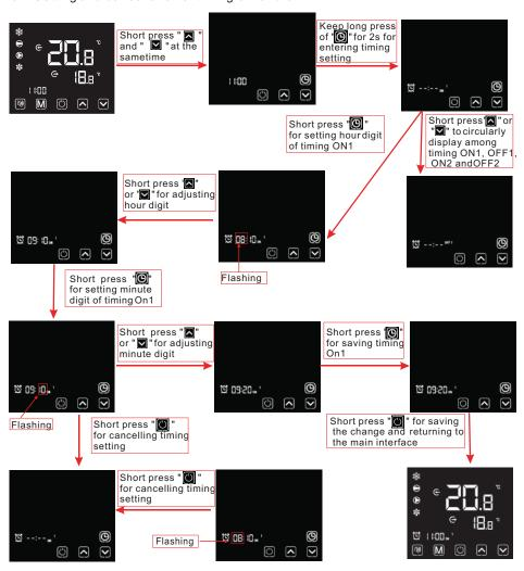
Notes: If there is no operation for 20 s, the system will automatically memorize user's setting, and return to the main interface; If the timing symbol and entire time digits flash at the same time, click " ror returning to the main interface.
