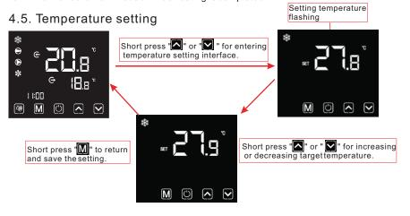
Notes: Under the temperature setting interface, if short press" [ ] ", the system will return to the main interface without any changes saved; If there is no operation for 5 s, the system will automatically memorize user?s setting, and return to the main interface.
