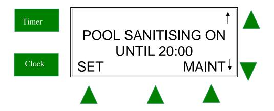
Press the **SET** button to change the chlorine output and the pH of your Pool
