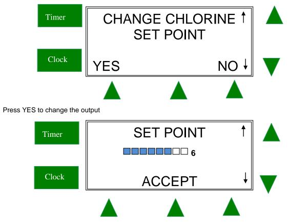
Use the up and down buttons to change the Set Point between 0 and 8. 0 chlorine output should only be used when there is no salt in the water. In summer, the chlorine should be set between 6 and 8 and you should regularly check your chlorine level in your swimming pool to determine if the output should be increased or decreased. Rely on your pool professional for advice on the recommended chlorine level in your pool.
