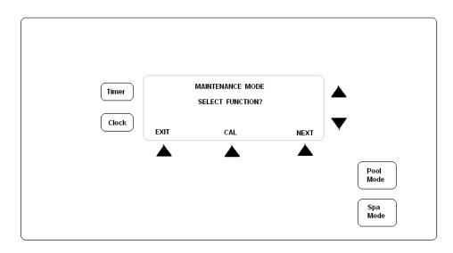
3. Select CAL option. Then select either PH or ORP calibration based on the option provided.
