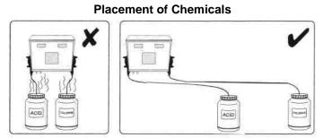
\*\*\*Chemicals MUST be stored apart in accordance with Relevant Standards and Dangerous Goods Codes. Consult your authorized builder or pool shop technician for advice. Chemicals must be at least 1 metre horizontally from control unit in a well ventilated area to avoid corrosive damage.
