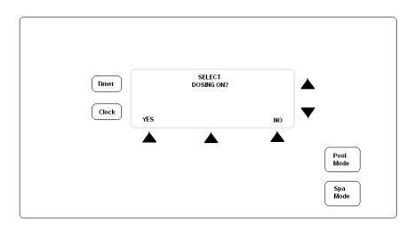
4. Select YES. You will be give the option to dose either Acid or Chlorine, pick the one you are wishing to dose. You will then need to set the dosing time/quantity using the up and down arrows to the right of the screen. You can choose to dose by volume of liquid or time period. Once you have set the volume/time to be dosed, select ACCEPT.
