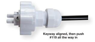
**Step 6.** Tighten #128 Cable Nut on the cable. This must be done tight enough to ensure the Quick-Connect Plug will not leak. You will need to hold the hexagonal area on the #120 Connector Housing with multi-grips or shifting spanner in order to tighten the 128 Cable Nut tightly.
