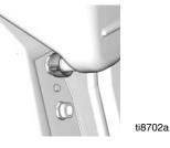
4. Loosen and remove 2 knobs (14) on sprayer handle (12).
