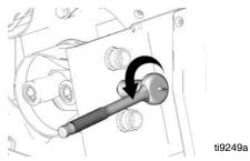
5. Grab pump hose (16) from side of unit and remove pump hose by hand.
