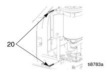
10. Slide motor tray (32) out of slots in base (2) to remove motor and tray from sprayer.
