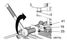
8. Feed wires and motor fuse through zip tie and lock into place.
