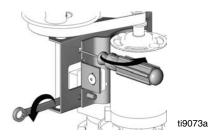
Once the motor is in place, you can test the belt to make sure it is properly tightened. When you push on the belt (24) with one finger it should move no more than 1/4 in. If it moves more than 1/4 in., go back to step 8 and re-tighten the belt.
