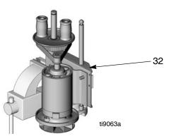
Use 9/16 in. wrench to loosen two mounting screws
