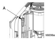
To remove the motor fuse, press down on the round center cover (C) and turn it counterclockwise.
