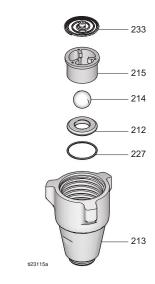
12. Install intake valve on cylinder. If a wrench is used torque as follows:
