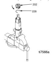
2. Unscrew intake valve from cylinder.
