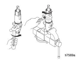
13. Torque packing nut (202) as follows:
