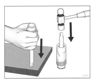
5. Unscrew piston valve from piston rod. Clean and inspect parts. The piston has a special thread locking/sealing patch. Do not remove the patch. The patch allows four disassembly/assembly procedures before it is necessary to apply medium strength threadlocker to the threads.
