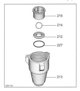
10. Install intake valve on cylinder. If a wrench is used torque to  $60 \pm 5$  ft-lb (81  $\pm$  7 N·m).
