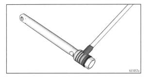
7. Grease top inch or two of piston rod that will go through the cylinder throat packings.
