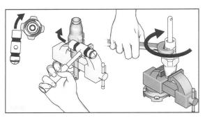
Disassemble intake valve. Clean and inspect o-ring (227). NOTE: A pick may be required to remove o-ring.
