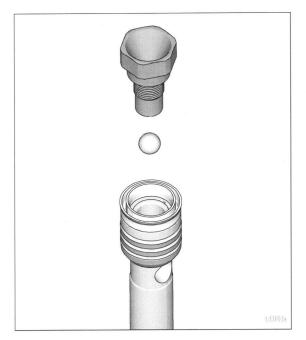
3. Tighten piston valve to piston rod. torque piston valve to 27 ± 3 ft-lb. (37 ± 4.1 N•m).
