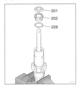
2. Unscrew intake valve from cylinder.
