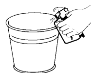
Trigger lock in locked position.
