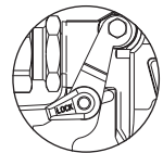
Trigger lock in locked position.
