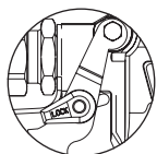
Trigger lock in locked position.
