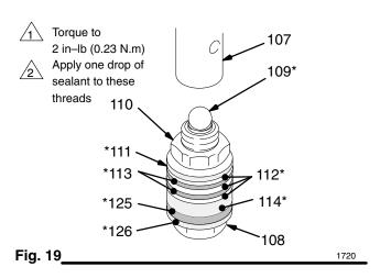
**NOTE:** Note the alignment of the piston (108) to the nut (110). Maintain this alignment through Step 8.
