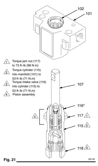
14. Place the ball guide (120), stop pin (122) and ball (121\*) in the cylinder (115). Screw the intake valve into the cylinder and torque to 53 ft-lb (71 N.m). This will also properly torque the cylinder into the manifold. See Fig. 22.
