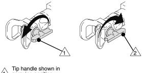
Tip handle shown ir spraying position.
