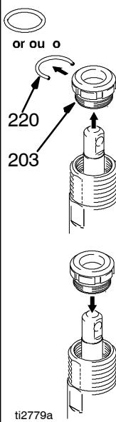
Remove throat nut spacer (220) when pump packings begin to leak after much use. Then tighten packing nut down until leakage stops or lessens. This allows approximately 100 gallons of additional operation before a repacking is required.
