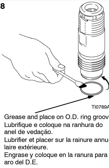
Grease and place on O.D. ring groove
