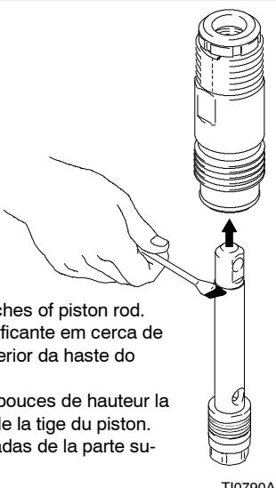
Grease top two inches of piston rod.
