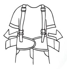
**STEP 2:** To tightern belt, grasp outer elastic bands and pull forward.
