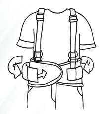
STEP 3: To fasten, attach outer elastic bands to the front of the belt.
