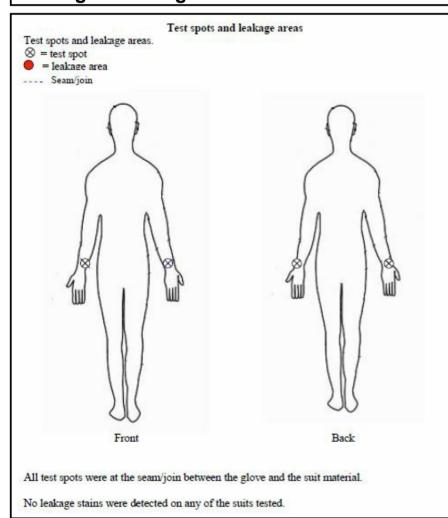
Leakage results in terms of area of total leakage stain(s) on the dosimeter suit as a ratio of the calibration stain are shown in the following table:
