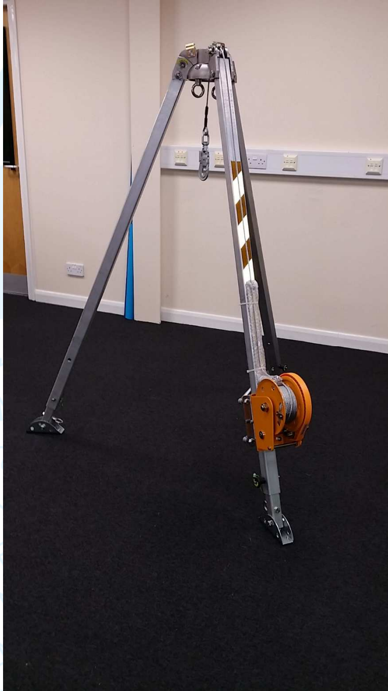
Figure 1 – Tripod and winch described as “HD-240”
