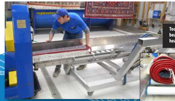
Using standard 100 PSI compressed air, any size rug is easily lifted from the floor with a single switch. It is then easily transported to the exact height of any Centri-Maxx centrifuge.
