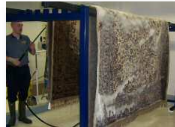
In addition to drying, the Quick Rack System can also be used for special wash processing while rugs hang.
