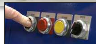
Fingertip controls are provided for stop, start, direction and rotation speed.
