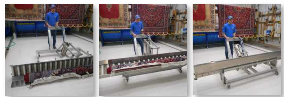
Using standard 100 PSI compressed air, any size rug is easily lifted from the floor with a single switch. It is then easily transported to the exact height of any Centri-Maxx centrifuge.
