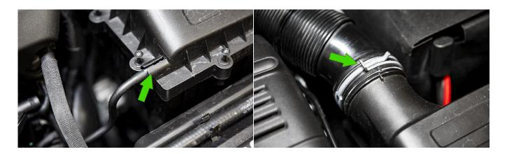
Remove the air filter then locate and remove the two (2) bolts using a T25 torx on either side of the upper air box inlet cover.
