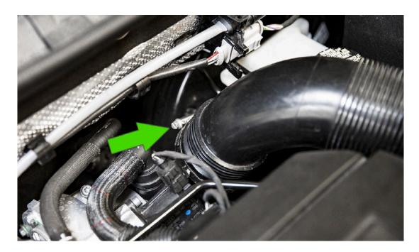
Install the MODE silicone inlet coupler and secure it tightly in place with hose clamp. Install larger upper stainless hose clamp and leave loose to allow fitment of the new MODE aluminium inlet pipe.
