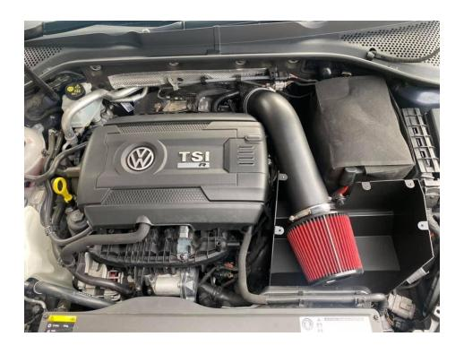
Install MODE heat shield lid and re install remaining OE Parts to complete installation.
