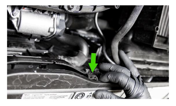
Pull up on the airbox base to release from the 3 grommets and completely remove it.
