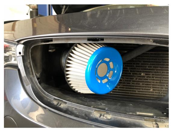
Test fit Kidney Grille without completely clicking into place. Once happy with position tighten clamps. If adjusted and fitted correctly the intake will not be touching anything.
