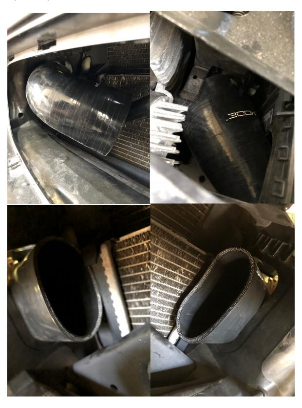
Install MODE Air+ Filter onto Velocity Stack and loosely fasten clamp.
