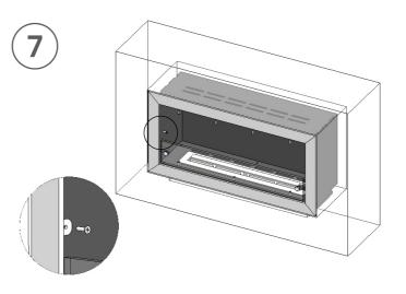
Using the screws you have removed in step 2 above, fix the frame (frames if the layout of the fireplace is open to more than one side) from the inside to the chassis of the fireplace. The frame is supposed to be flush with the surrounding wall surfaces. Make sure there is a 5mm gap between the frame and the surrounding wall material all the way around.
