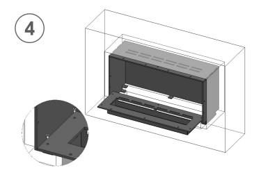
Lift the base plate into the fireplace taking great care not to scratch the paint on the sides and back. Use the screws you have removed in step 2 above and fix the base plate to the chassis of the fireplace.
