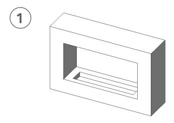
Check that the dimensions of the cut-out are in accordance with the technical drawing provided with the fire-place. All corners of the cut-out must be in a 90° angle and all surfaces in level.
