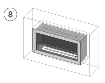
The fireplace is now installed and ready for use. Fill the burner up to the max. level indicator and light it with a long lighter or fireplace match.
