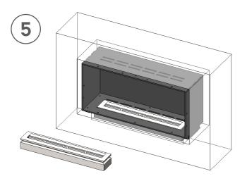
Place the burner inside the safety chamber and place its slider lid on top of the burner opening.
