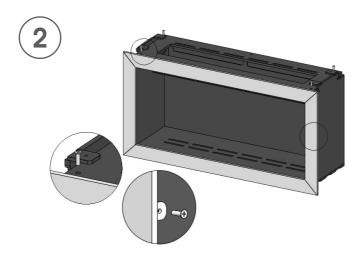
The decoflame® Orlando has been assembled with its frame and its base plate fitted upside-down in order to stabilise the fire during transit. Unscrew the screws that hold the frame and the base plate fitted to the chassis of the fire. Keep the screws as you will need them in step 4 and step 7 of the installation!
