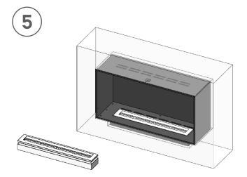
Place the burner inside the safety chamber and place its slider lid on top of the burner opening.
