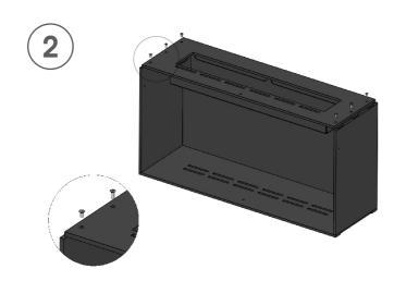
The decoflame® Montreal has been assembled with its base plate fitted upside-down in order to stabilise the fire during transit. Unscrew the screws that hold the base plate fitted to the chassis of the fire. Keep the screws as you will need them in step 4 of the installation!
