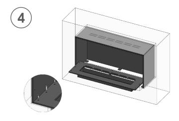
Lift the base plate into the fireplace taking great care not to scratch the paint on the sides and back. Use the screws you have removed in step 2 above and fix the base plate to the chassis of the fireplace.
