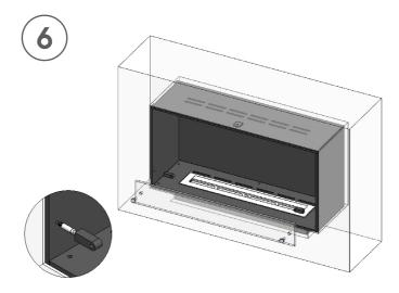
Take the stainless steel threaded bolts (male parts) from the little plastic bag and screw them into the holes at the lower front of the sides of the chassis of the fireplace. Push the glass holders (female parts) over the ends of the threaded bolts. The threaded hole at the other end of each glass holder is facing to the front. Fix the glass holders in this position by tightening their hexagon set screws with an allen key.
