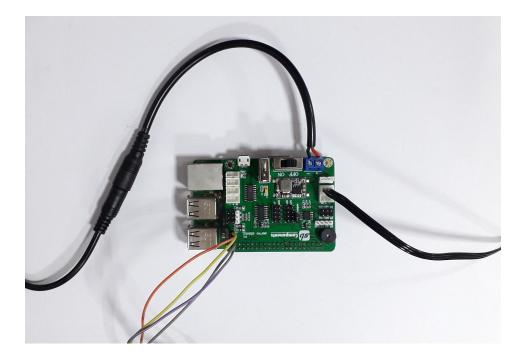
Or you can also use USB serial communication, USB communication will work the same way as GPIO. With USB serial communication it's up to you if you want the Servo Shield stacked over the Raspberry Pi or not.
