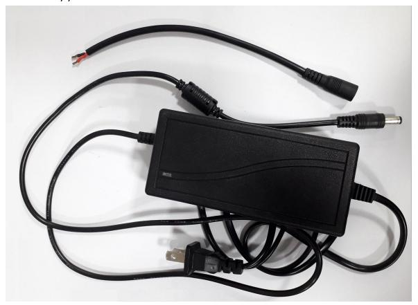
Connect the two-wire connector with the blue pvt connector on servo shield(make sure the polarity is correct). Once the connection is set up connect your servo motor's wire into the white connector
