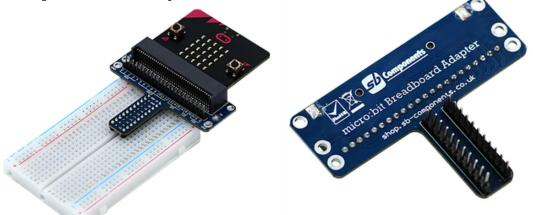
In order to facilitate the wiring of micro:bit development board, we specifically design this T-type breadboard adapter. It can be connected to the micro bit development board easily, then can be directly plugged onto the breadboard. You can use it in your experiments, simply wire it up on the breadboard using breadboard jumper wires, pretty easy and convenient.
