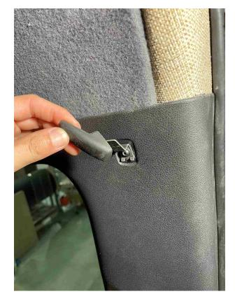
1. Begin by removing the rubber covers from the coat hooks and, if present, the bolt covers on the grab handles.
