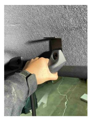
4. Next, reattach the coat hook along with the B pillar bracket.
