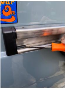
Step 5. Install end clip back into track end.
