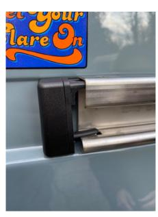
Step 6. Remove tape tabs, snap trim in place and press.
