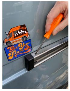
Step 4. Separate the end cap from the track end clip
