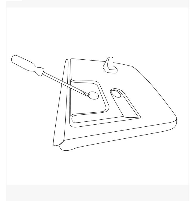
Step 2: Install the mounting tabs into the roof mounting holes, and it is recommended to apply sealant between the mounting tabs and the roof.
