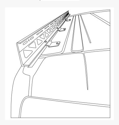
Step 5: Securely bolt together the front and rear sections of the sidewalls using the included tab and hardware.
