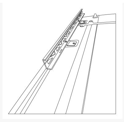
Step 4: Install the rear section of the side wall onto the mounting tabs using the provided hardware.
