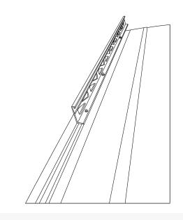
Step 3: Install the rear section of the side wall onto the roof rail.
