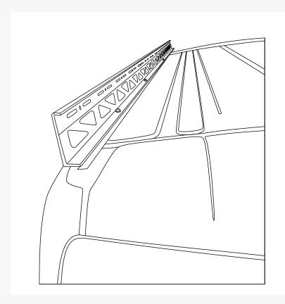
Step 4: Securely bolt together the front and rear sections of the sidewalls using the included tab and hardware.
