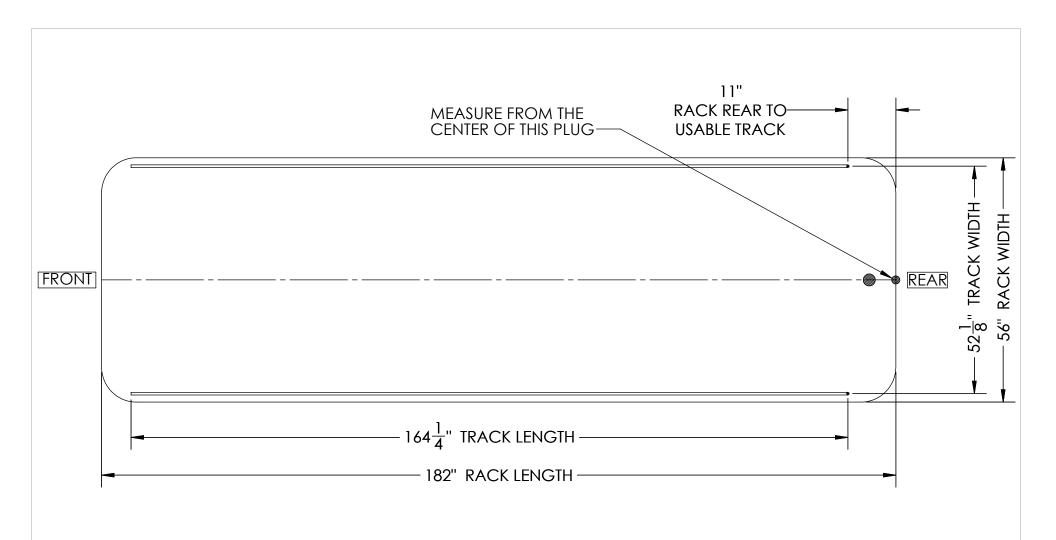
DRAW LINES WHERE YOU WANT WELDED UPPER LOOP CROSSBARS LOCATED WITH A DISTANCE FROM THE BACK OF THE RACK. INDICATE MODEL, DIMENSIONS AND DESIRED LOCATIONS OF SOLAR PANELS TO ENSURE FITMENT.
