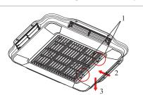
• Remove the air filter from the plenum by pushing both tabs inwards and then downwards.
