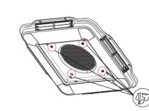
• Attach the plenum assembly to the plenum mounting bracket by engaging the two parts.
