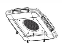
• Fix the plenum assembly on the plenum mounting bracket with four ST4×19 pan
